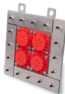
KRASO® Cable Penetration KDS 150 FL/ZA as multiple wall penetration - with fixed-loose flange and exterior protrusion flange FDS 150, for dowel-fixing (special production)
