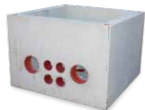
KRASO® Pump Sump - concrete - Special internal dimensions approx. 100 x 100 x 80 cm, made of waterproof concrete, with 12 cm thick, steel fibre reinforced wall and base plate (20 kg per cbm). Connections: 2 x DN 200, 4 x DN 110, 1 x DN 110 in the bottom, total weight: approx. 1.5 t
