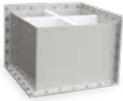
example 80 x 80 x 60 cm with flange plate for pressing on, for the sealing on an existing concrete wall, incl. EPDM supplement, drill holes Ø 12 mm to clamp and KRASO® PU 50 for adjusting unevenness of the existing wall
