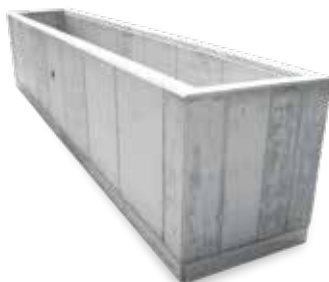
KRASO® Pump Sump - concrete - Special internal dimensions approx. 100 x 750 x 140 cm, made of waterproof concrete, with 20 cm thick, steel fibre reinforced wall and base plate (20 kg per cbm) and 1 x pipe connection DN 110, without rebar connection, without joint tape, total weight: approx. 17.5 t
